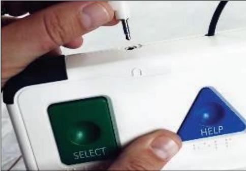
2. Right port for any dual-switch input device – such as sip and puff device
