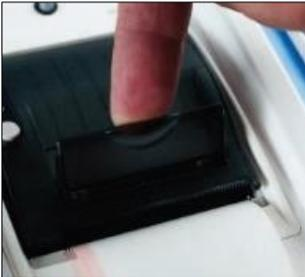
1. To open the paper compartment, pull the lever on the top of printer cover towards you and lift it up.
