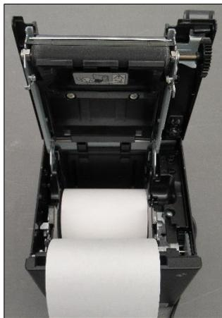
2. Remove the adhesive portion of the new roll. Insert the roll in an “under” format so it rolls up from the bottom.
