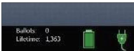
15. Record the zero Ballots count shown at the bottom of the screen on the applicable line of the **Register of Official Ballots** form, which is inside the Clear Bag.
