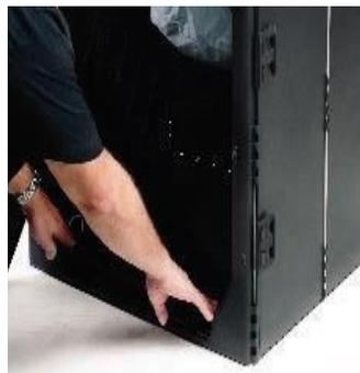
Unlock the large front door with the round gray key. Use your foot or hand to firmly press on the 'Press Here' points to lock the floor into place.
