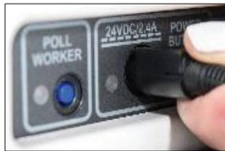
8. Plug the round end of the cord, flat side up, firmly into the back of the case in between the blue poll worker and red Power Buttons. Plug the power cord into a wall outlet. Open the case and secure the lid again.
