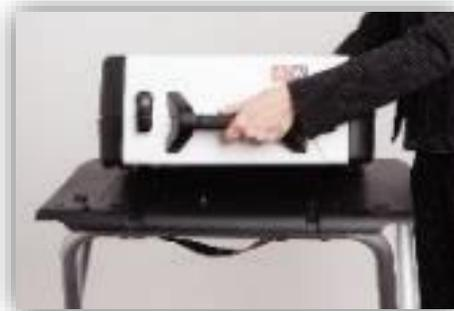
2. Place a Duo, cases marked with the letter D, on each of the trays, with the handle on the case facing the same direction of the handle that is underneath the table tray, and aligning the footpads with the indentions.
