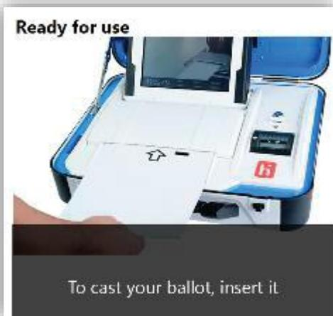
18. The tablet will display 'Ready for use' at the top and 'To cast your ballot, insert it' at the bottom of the screen.
