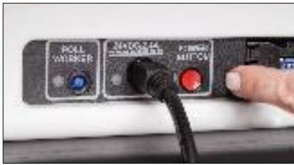
12. Press the red Power Button on the back of the case to power on the Scan. It is normal for the tablet screen to go black for a short period.
