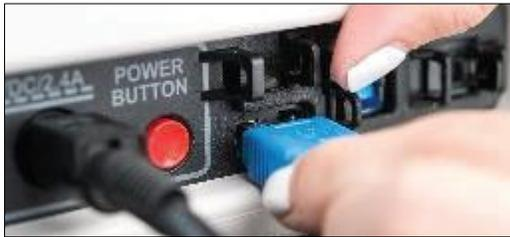
11. Plug the device into the back of the Duo, in the port between the red Power Button and the verity cables. If the port is not visible, lift the cover up. Open the cases and secure the lids again.
