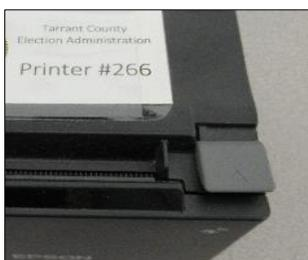
1. To open the lid of the stationary printer, lift the lid from the gray lever. Remove the empty spool.
