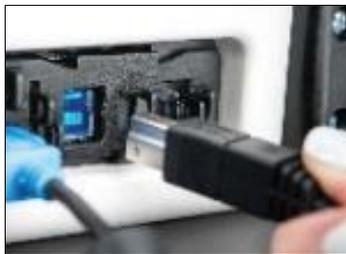
8. From the supply box, grab a Verity Cable, long black cable with matching inner ends, and plug either end, smaller side up, firmly into the back of the case underneath the word Verity Cables. If the ports aren't visible, slide the cover to the right. Open the case and secure the lid again.
