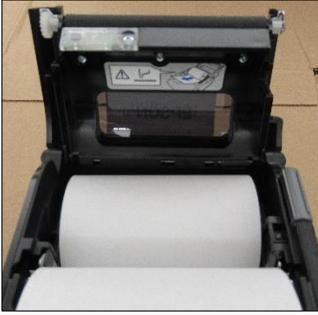
4. Remove the adhesive portion of the new roll. Insert the roll in an “under” format so it rolls up from the bottom.
