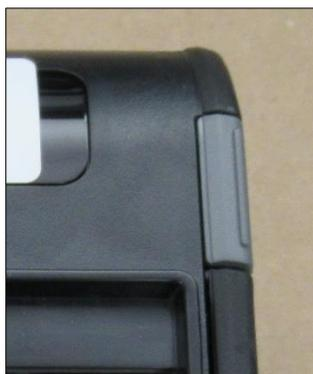
3. To open the lid of the portable printer, push in the gray button. Remove the empty spool.
