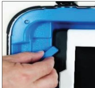
12. Use the round key color coded in black, insert it into the keyhole near the blue door and unlock it by turning the key to the left while leaving the key in place. Raise the blue latch on the upper left corner of the tablet.
