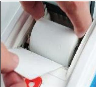
2. Place the new paper roll in an “under” format so it rolls up from the bottom.
