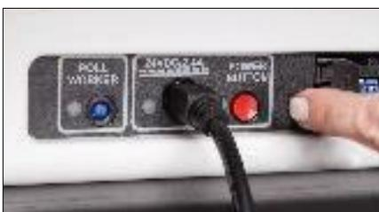
13. Press the red Power Button on the back of the case to power on the Controller. It is normal for the tablet screen to go black for a short period.
