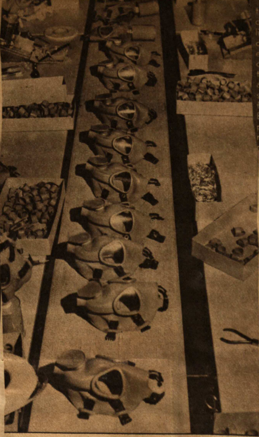
A ROW OF MASKS with eye pieces and breathers attached are conveyed to the section where chemical can and attachments are added.
