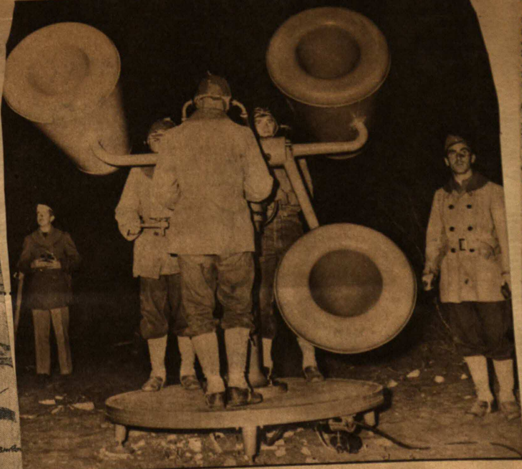
THE SOUND LOCATER goes into action as "enemy" planes approach. The operators are Lieut. Devine (left), Pvts. Pecoraro, Sawyer, Parker, and Sgt. McCarthy (right).
